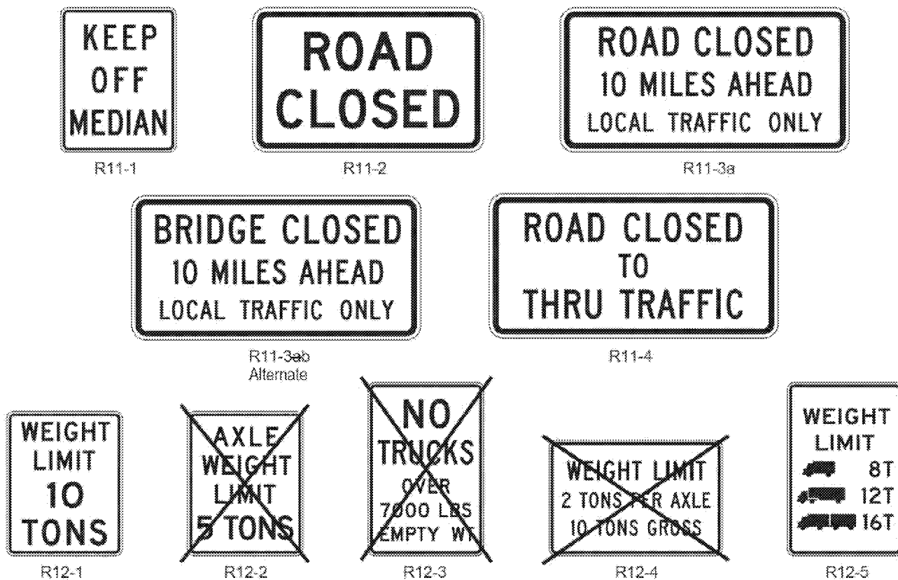
Figure 2B-29. Road Closed and Weight Limit Signs
