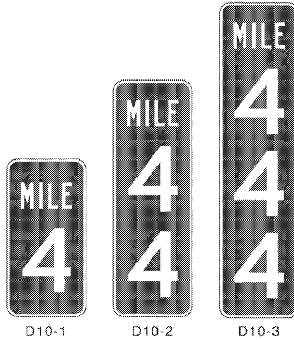
Figure 2H-2. Reference Location Signs
