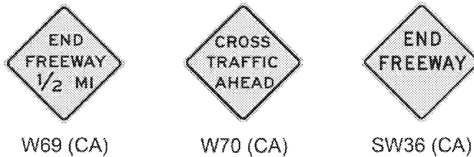
Figure 2C-9 (CA). Intersection Warning Signs and Plaques
