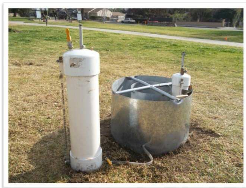
Double Ring Infiltrometer (ASTM D3385) Test Setup
