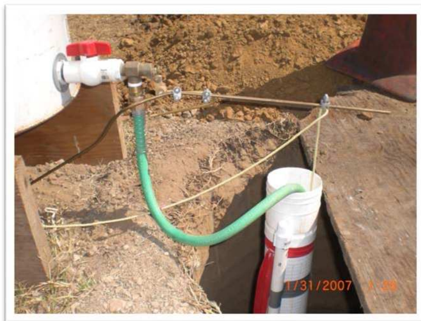
Well Permeameter (USBR 7300-89) Test Setup
