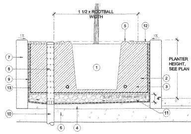
PIPE WRAPPED IN DRAINAGE SOCK WITH REMOVABLE THREADED P.V.C.
