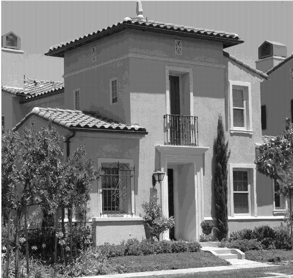
Example - Multiple Family Building Articulated with a Lower Height Element, Wrought Iron and Trim Details, Balcony and Banding Details.
